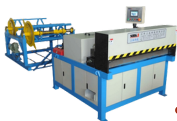
DUCT AUTOMATIC LINE III
